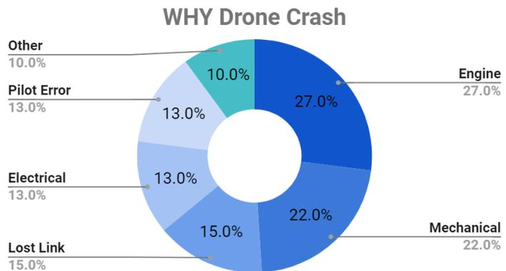
Then we have that 13% of the crashes are attributed to electrical failures. These include the failure of onboard power generators and various servomotors as well as the failure of wiring and cables bringing power to particular pieces of equipment.
