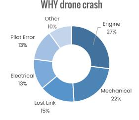
Then we have 13% of the crashes (for which we have cause details) are attributed to electrical failures. These include the failure of onboard power generators and various servomotors as well as the failure of wiring and cables bringing power to particular pieces of equipment.
